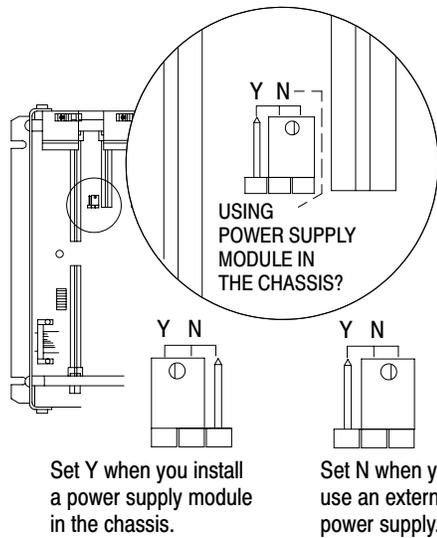
1. Locate the chassis configuration plug (between the first two left most slots of the chassis).
