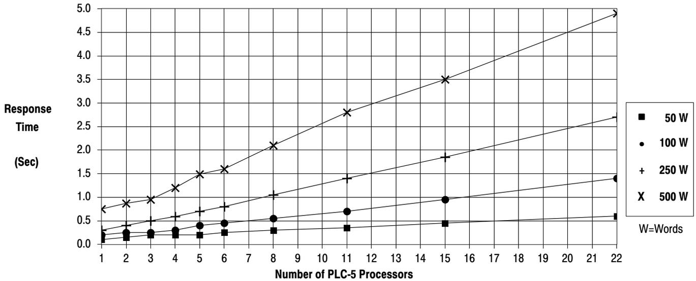
Figure 5.6 shows the effect of a programming terminal on message response time under various configurations.
