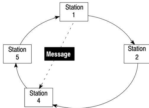
Station 1 has the token. Only the station that has the token can send a message. Station 1 sends the message to station 4. Now station 1 must pass the token on to the next highest station number, which is station 2.
