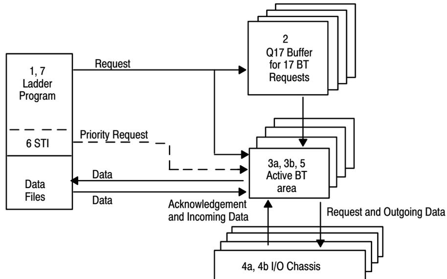
1. Ladder logic enables the block transfer.
