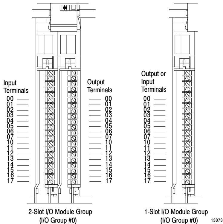
An **I/O rack** is an addressing unit that corresponds to 8 input image-table words and 8 output image-table words. A rack contains 8 I/O groups.
