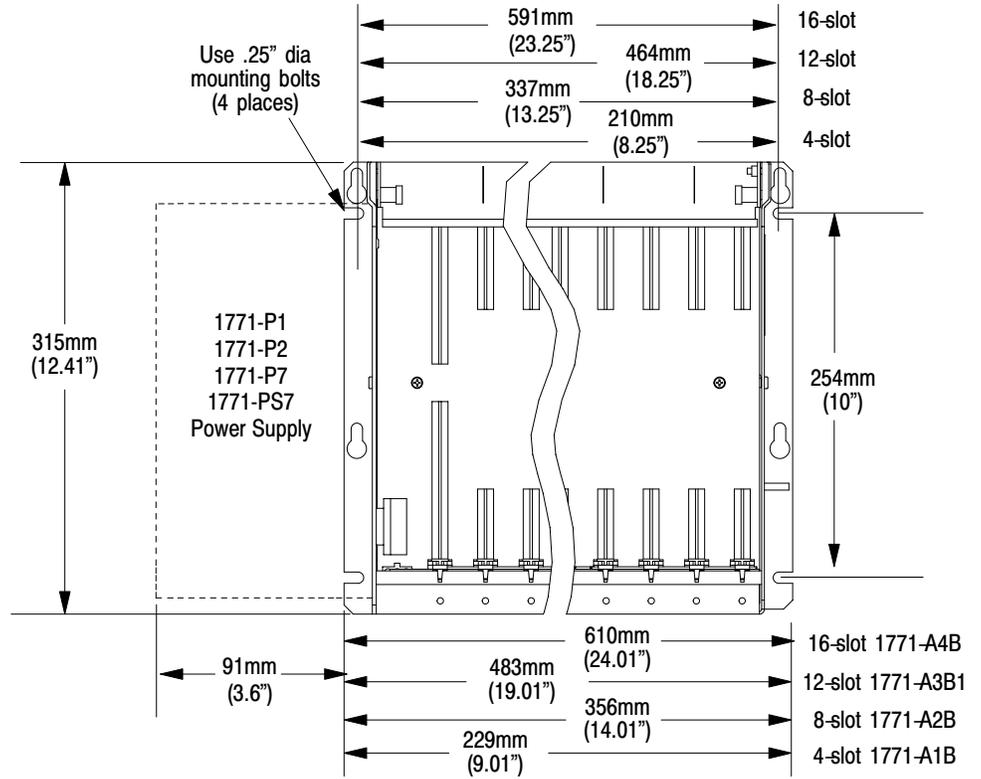
Clearance depth is 204 mm (8 in) for 8 I/O connection points per module.
