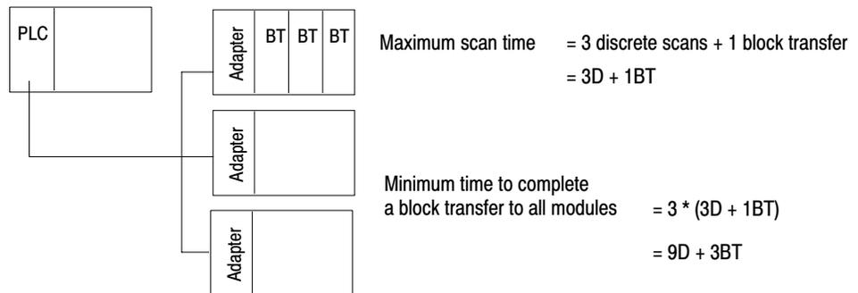
If you place the three block-transfer modules in different racks, however, you can block transfer to all three modules in one I/O scan. To optimize your system layout for **block-data transfers**, use an arrangement similar to the following:
