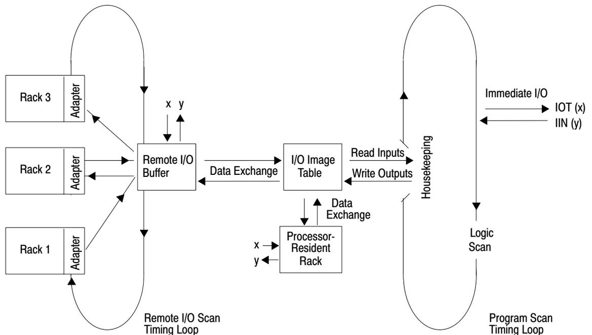
During the housekeeping portion of the program scan, both the remote I/O buffer and the processor-resident rack are updated. Remember that the I/O scanner is constantly updating the remote I/O buffer asynchronously to the program scan.
