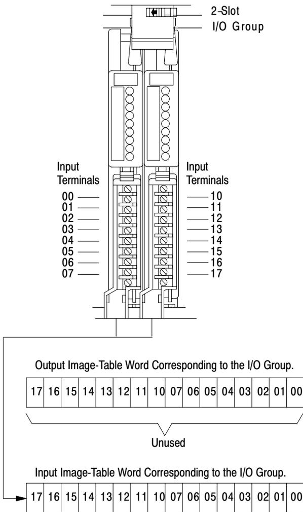
This I/O group uses 16 bits of the input image table.
