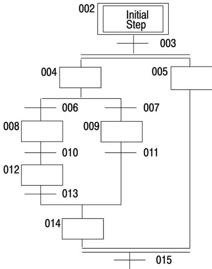
Each step corresponds to a control task (displayed as a box); each step is related to a program file that contains the logic for the associated control task. Each transition (displayed as a horizontal line) examines conditions, specified in an associated program file, that determines when the processor can continue to the next task.
