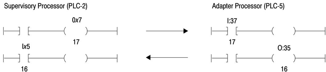
When the supervisory processor sets its output file bit  $0x:7/17$ , input file bit  $I:37/17$  in the adapter-mode processor is automatically set. In the same way, when the adapter-mode processor sets output file bit  $O:35/16$ , input file bit  $Ix:5/16$  in the supervisory processor is automatically set.
