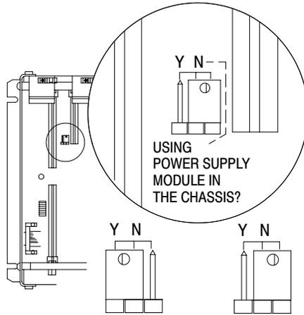
Set Y when you install a power supply module in the chassis.
