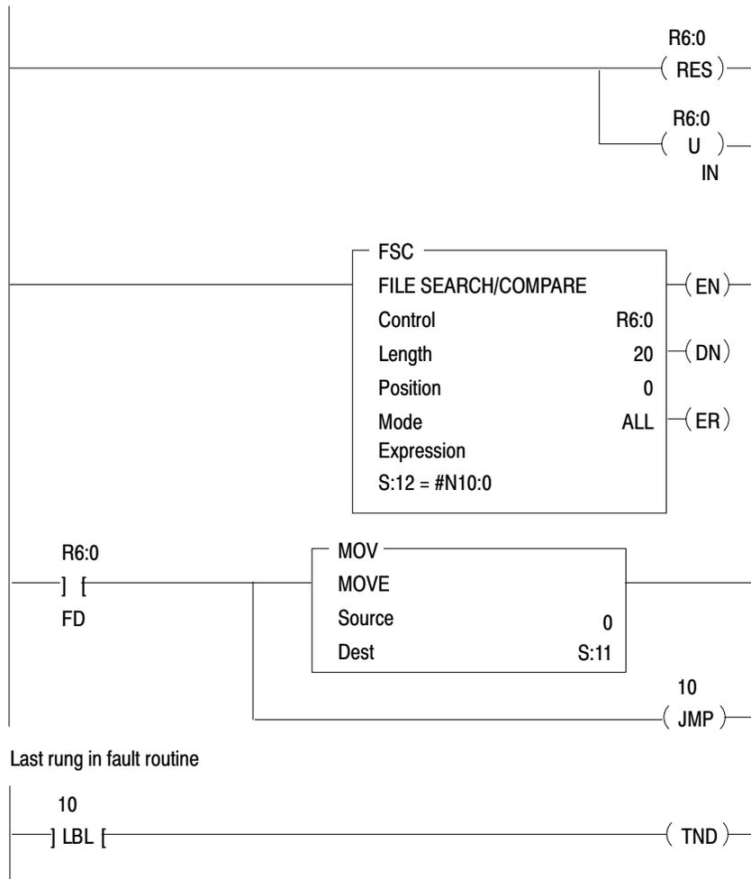
The processor completes the scan of the fault routine. If the routine clears S:11, the processor returns to the program file and resumes program execution. If the fault routine does not clear S:11, the processor executes the rest of the fault routine and goes into FAULTED mode.
