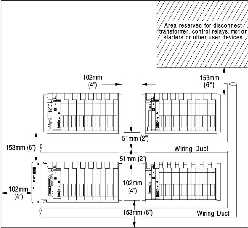
**Minimum spacing requirements for a remote I/O chassis:**
