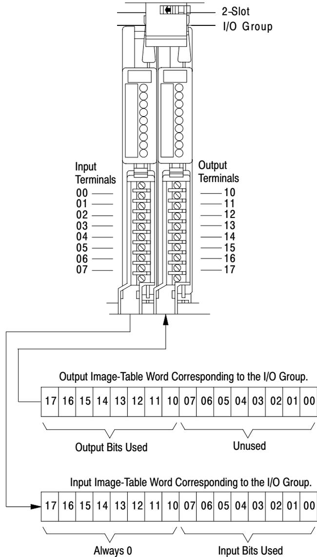
This I/O group uses 8 bits of the input image table and 8 bits of the output image table.
