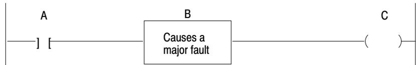
In the example in Figure 7.3, the processor runs the fault routine after detecting the fault. If the fault routine resets the faulted bits, the processor returns to the next instruction in the program file that follows the one that faulted and outputs on the remainder of the rung.
