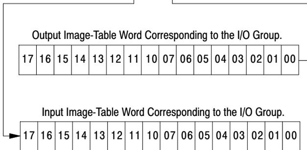
This I/O group uses 16 bits of the input image table and 16 bits of the output image table.
