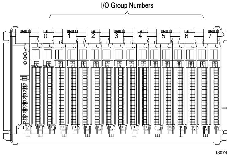
Depending on I/O chassis size and I/O group size, an I/O rack can occupy a fraction of an I/O chassis, a full I/O chassis, or multiple I/O chassis.
