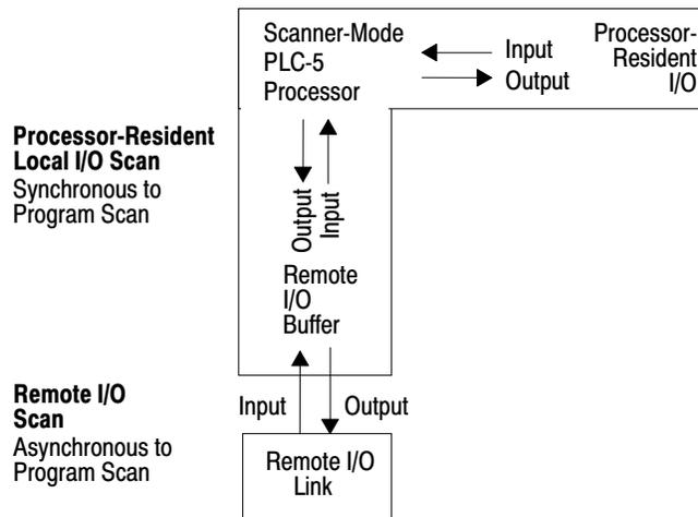
The scanner-mode PLC-5 processor can also:
