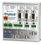
The Anybus ProfiHubs can be detected by the ComBricks, which allows you to view every channel individually via the integrated web server
